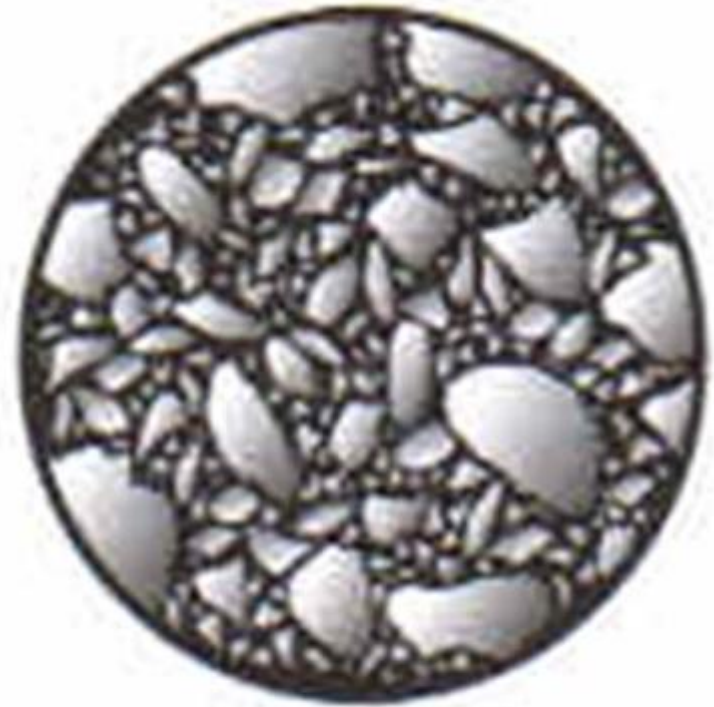
MMA typu AC (Asphalt Concrete)
