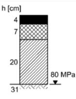
asphalt concrete wearing course asphalt concrete binder course
